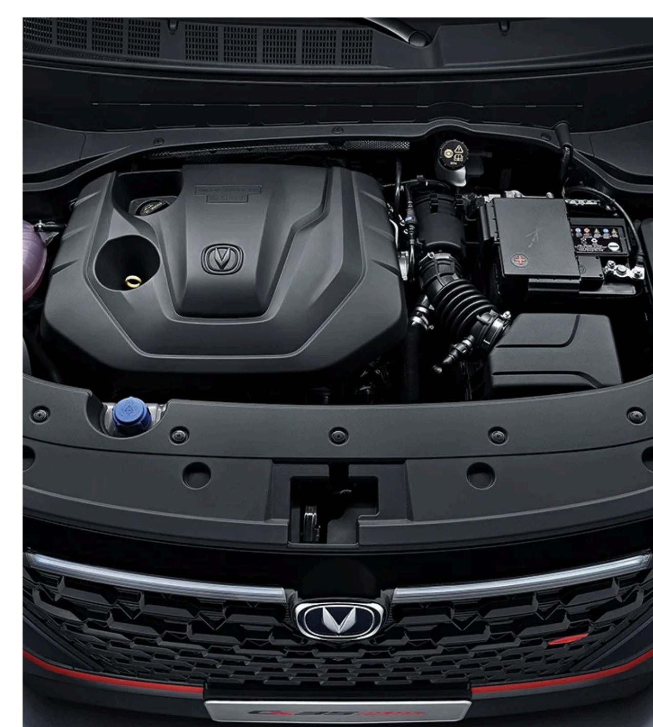
1.4 Litre Turbo Engine (158 HP)
